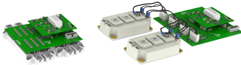
Pic 3: Adapter boards for spring (left) and wire (right) contacted boards
